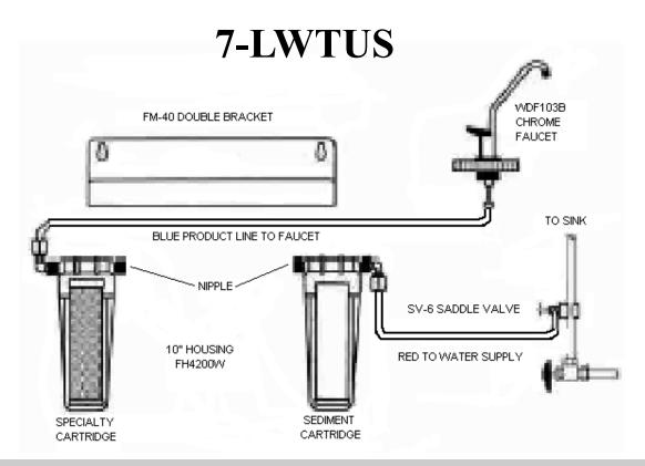
This system requires regular replacement of the filter cartridges to maintain proper operation. The maximum life of a cartridge is three months. Individual water conditions may effect change frequency.
