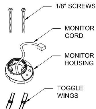
4. Feed the Monitor Cord through the 1 1/4" diameter Monitor Housing opening so that it is positioned above the Monitor Housing.
