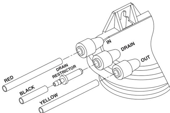
2. Locate the  $\frac{1}{4}$ " Red Feed Water Tubing. Remove the red plug from the fitting labeled "In" on the manifold and insert the tubing. Reference the special supplement sheet in the carton for proper connection of all tubing and removal of plugs. Run the tubing along its course to the Feed Water Saddle Valve, trim to length. (Refer to Fig. 1).
