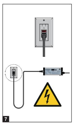
Plug the electronic ballast controller into the GFCI outlet and power-up the system.
