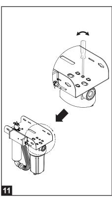
Vent to purge air and to complete the disinfection procedure.
