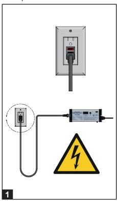
Ensure the electronic ballast controller is plugged in for entire disinfection process.
