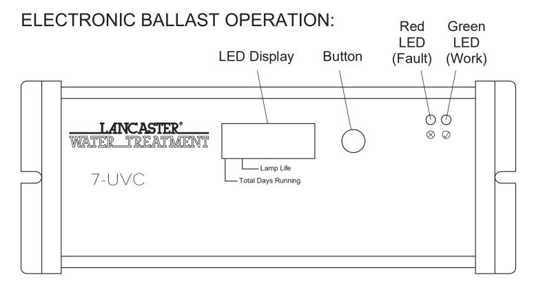
The 7-UVC Electronic Ballast (a.k.a. EPS-Electronic Power Supply or simply "controller") is equipped with visible and audible operation indicators:
