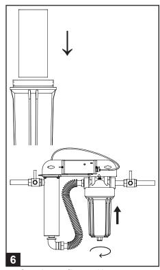
Open the new filter cartridge wrap and discard wrap. Insert the new filter cartridge into the sump housing and connect to the unit using the sump spanner wrench.
