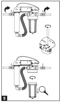
With valves closed, vent pressure and remove sump housing using sump wrench.
