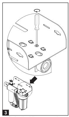
Slowly and partially open vent to release the pressure from the filter.
