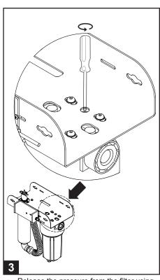
Release the pressure from the filter using the vent-valve on top of the filter head.
