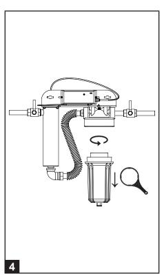
Remove sump housing using sump wrench.
