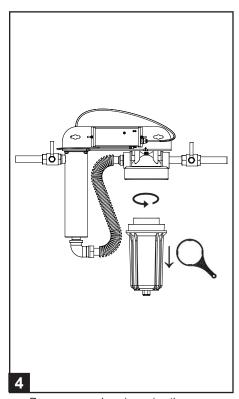
Remove sump housing using the sump spanner wrench.
