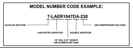
Congratulations on purchasing your new LANCASTER AERATION SYSTEM. When installed with a properly selected automatic backwashing filter, this system will provide a chemical-free method to reduce iron and hydrogen sulfide levels in your well water. For servicing and future inspection purposes, please file this booklet with your important documents.
