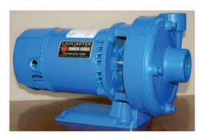
The back-pull-out feature allows the motor, motor adapter, seal, and impeller to be removed without disturbing pipe connections. Maintenance is therefore considerably simplified.
